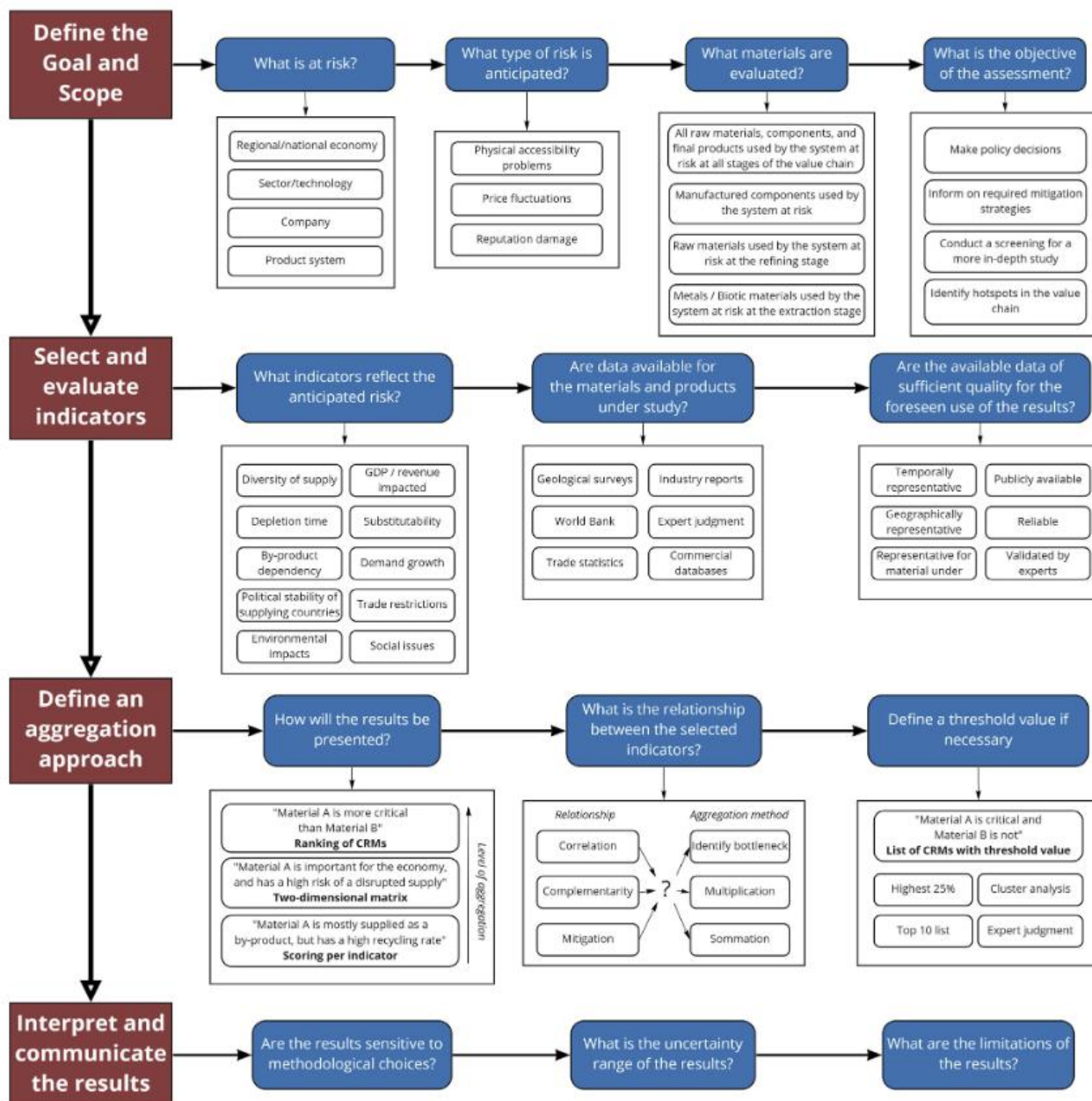
Figure 2. Step-by-step guidance for the design and communication of a criticality assessment, with examples of potential methodological choices (Helbig et al. 2021).
